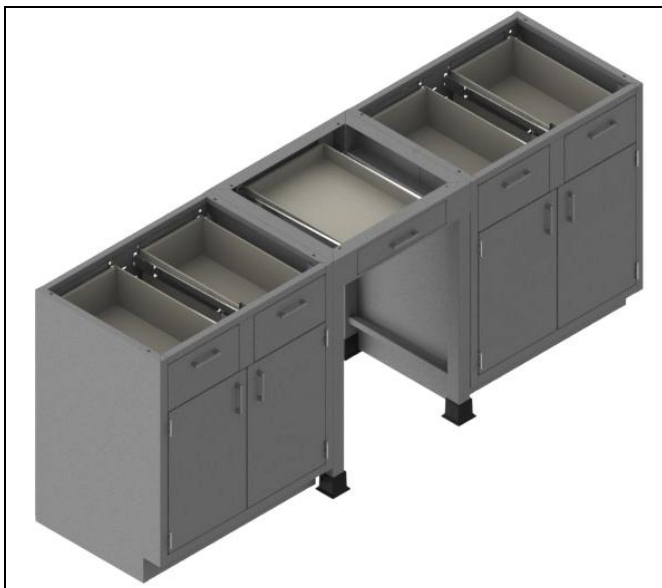
Steps C & D: Level apron and secure to adjoining cabinets; tighten the bolts to lock the legs in place .
